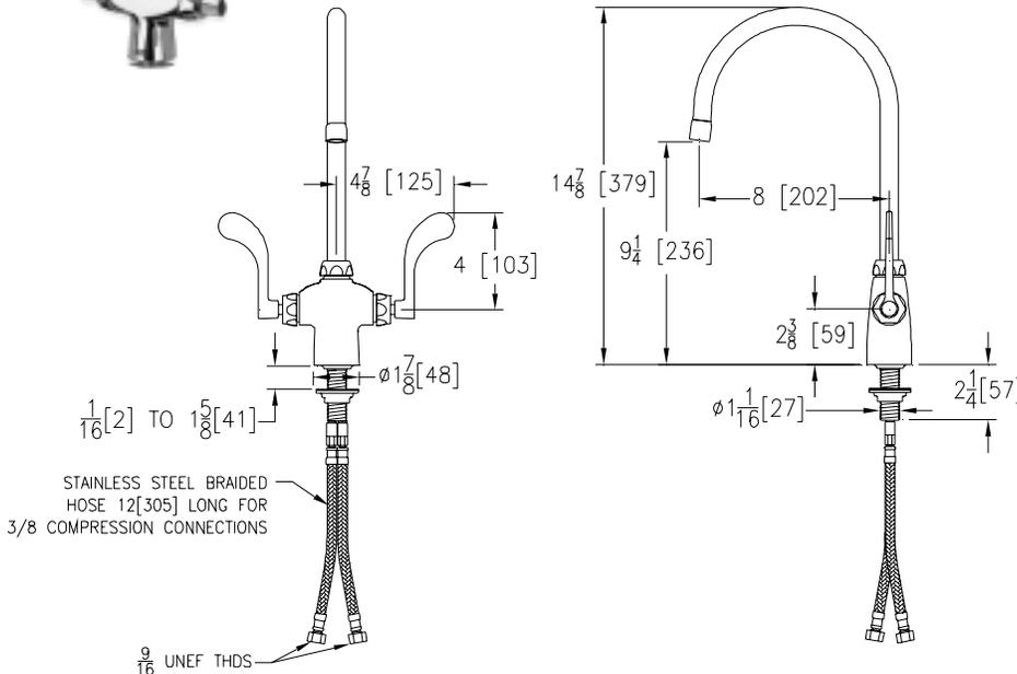
Zurn Lead Compliant\* "XL" products are a line of durable, high quality brass faucets and fixtures that are designed and manufactured to comply with state laws and local codes that mandate lead content levels. Zurn "XL" products are manufactured with \*not more than 0.25% lead content when used with respect to wetted surfaces of pipes and pipe fittings, plumbing fitting and fixtures: California Health & Safety Code § 116875; Vermont 9 VCA § 2470h
