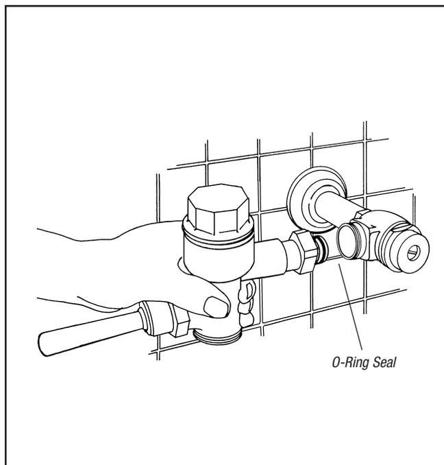
**2** Insert flush valve tailpiece into stop valve, being certain O-ring seal is in place. Wet seal with water to lubricate. Hand tighten locknut. Determine length of vacuum breaker tube required and cut as necessary. Assemble vacuum breaker tube assembly between flush valve and fixture spud.
