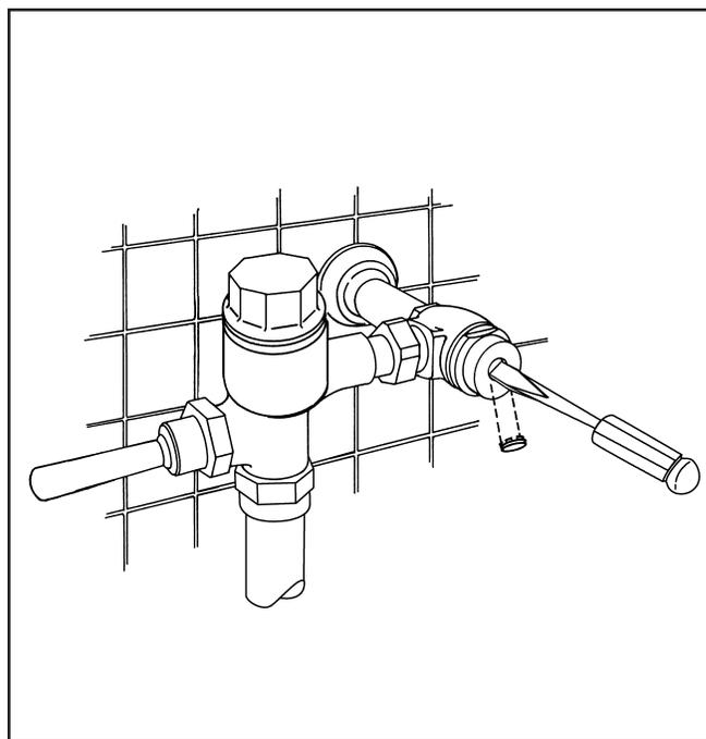
**4** Set flush valve for proper operation by adjusting stop valve. Stop valve adjustments can only be made by using the adjusting screw located behind the adjusting screw cover. (Water must be shut off at main supply valve if stop cap is to be removed.) Final setting should provide enough water flow to evacuate a closet fixture and should be such that a urinal fixture will not overflow when continually flushed. Secure adjusting screw cover.
