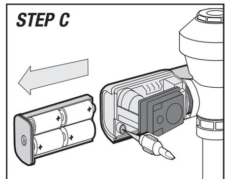
Sensor Adjustor Tool comes in a built-in storage pocket. Replace after use.
