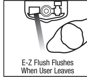
The E-Z Flush™ sends out a continuous infrared beam that is reflected back by the presence of a person in front of the urinal or toilet. The technology differentiates between someone walking past the unit or actually using the fixture. E-Z Flush models ZERK-CP and ZERK-CPM retrofit Zurn and Sloan valves. For Delaney valves, order model ZERK-CP-LY or ZERK-CPM-LY.
