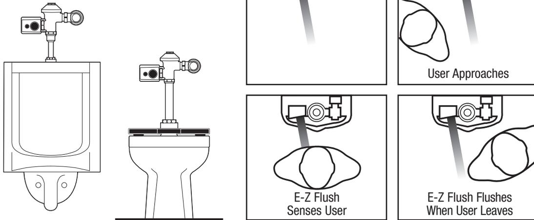
The E-Z Flush™ sends out a continuous infrared beam that is reflected back by the presence of a person in front of the urinal or toilet. The technology differentiates between someone walking past the unit or actually using the fixture. E-Z Flush models ZERK-CP and ZERK-CPM retrofit Zurn and Sloan valves. For Delaney valves, order model ZERK-CP-LY or ZERK-CPM-LY.
