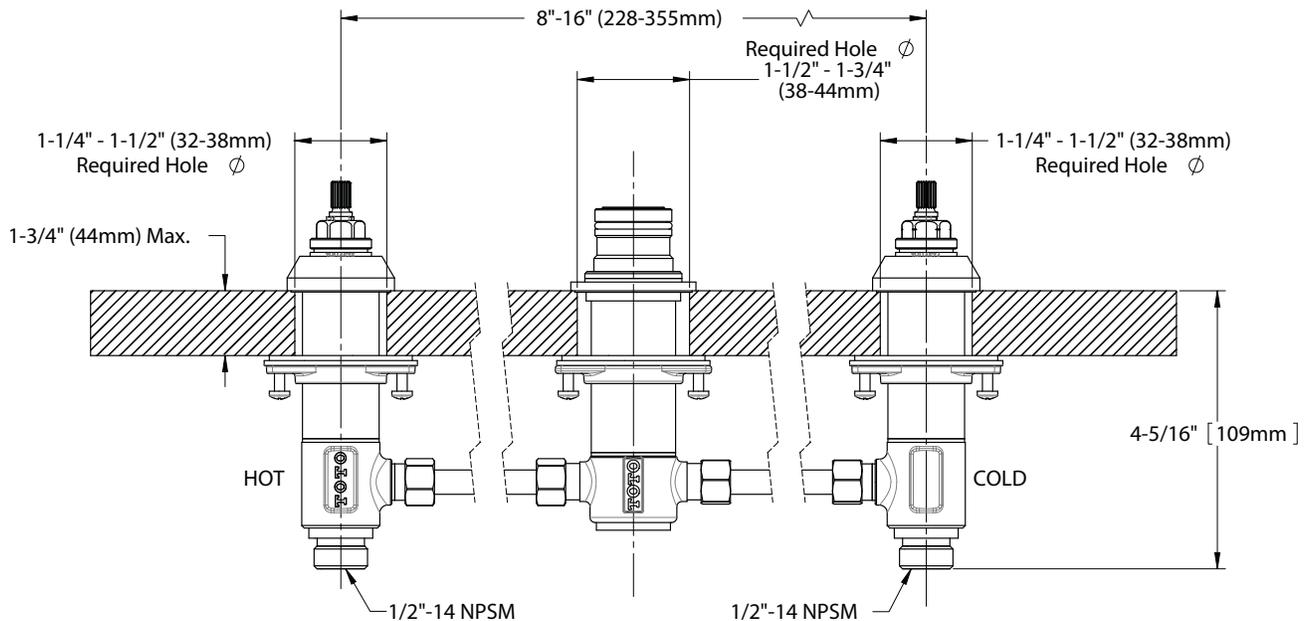
**Important Note:** This product must be installed after the deck or tub rim is finished.
