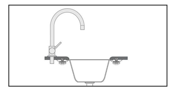
Caution: All installation types need to allow room for faucet installation. Ensure adequate clearance behind the basin for your faucet and backsplash, as well as the full range of motion for faucet handles and spouts.
