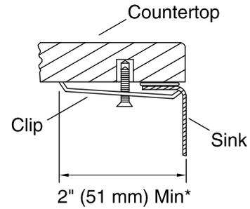
\* Allow clearance around sink rim for clip attachment.
