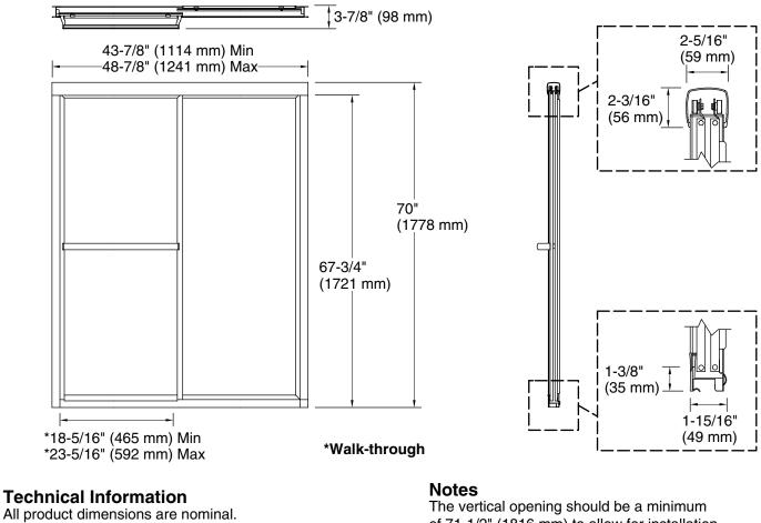
Installation type: For shower base installation Base-To-Wall 1/2" (13 mm) Radius – Max: The vertical opening should be a minimum of 71-1/2" (1816 mm) to allow for installation clearance.
