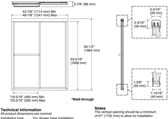
Installation type: For shower base installation Base-To-Wall 1/2" (13 mm) Radius - Max: Glass thickness: 1/8" (3 mm)
