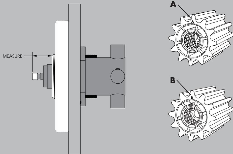
**5** Confirm that the Valve is in the off position. Insert Spine Adapter (1) over Kohler spindle (2), with the appropriate side "A" or "B" facing outward. (determined in Step 4). One set of splines on the adapter must be oriented perfectly vertical when installed, as shown below. Secure the Spine Adapter with the 8-32 X 7/8" Screw (3) provided.
