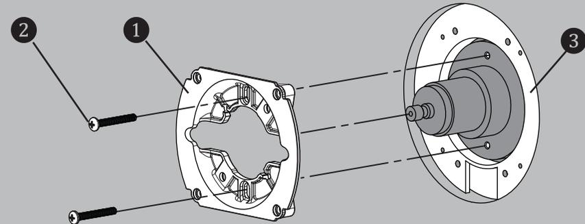
**NOTE:** Valve Mounting Plate (1) should sit flush upon Kohler Mounting Flange (3) when secured.
