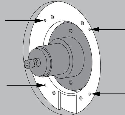
**2** Clean front surface of wall. Install Valve Mounting Plate (1) to existing Kohler Valve, using the 10-24 x 1-1/2" screws (2) provided. Take care to not over tighten mounting screws.
