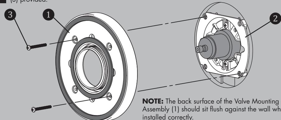
**NOTE:** The back surface of the Valve Mounting Plate Assembly (1) should sit flush against the wall when installed correctly.
