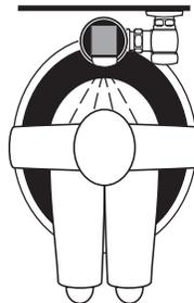
3. When the user steps away from the SOLIS® Sensor, the Sensor initiates an electrical signal that operates the Solenoid. This initiates the flushing cycle to flush the fixture. The Circuit then automatically resets and is ready for the next user.
