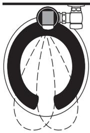
2. As the user enters the beam's effective range (15" to 30") the beam is reflected into the SOLIS® Scanner Window and transformed into a low voltage electrical circuit. Once activated, the Output Circuit continues in a "hold" mode for as long as the user remains within the effective range of the Sensor.
