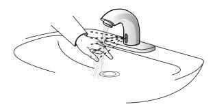
Place hands under faucet. Solenoid valve should "click," LED in sensor window should blink once and water should flow from the spout.
