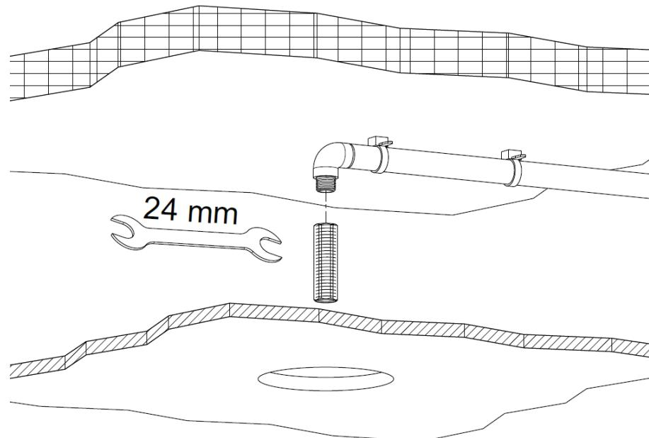
Then, screw hermetically the threaded connection using a 24 mm wrench together with hemp or similar materials.
