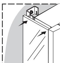
Align the edge of the side mirror behind the flange.
