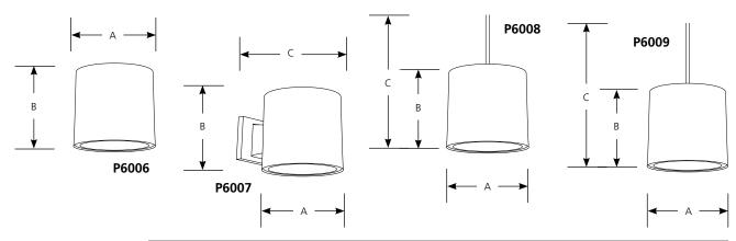
The P6000 Series LED cylinders are nominal 6" cylinders designed to be used with the P8071 series trims. Available in surface, wall, pendant, or cord mount, they provide a cost effective option for LED surface lighting. It is suitable for a wide varity of commercial, retail and institutional applications.
