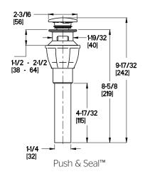
Ø1 Min to Ø1-1/2 Max. Deck Hole Openings
