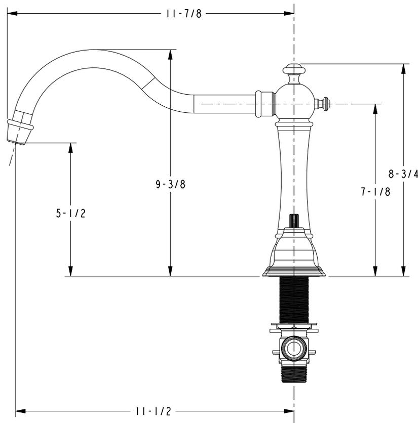
DIMENSIONS ARE IN INCHES AND AN APPROXIMATION OF A TYPICAL INSTALLATION
