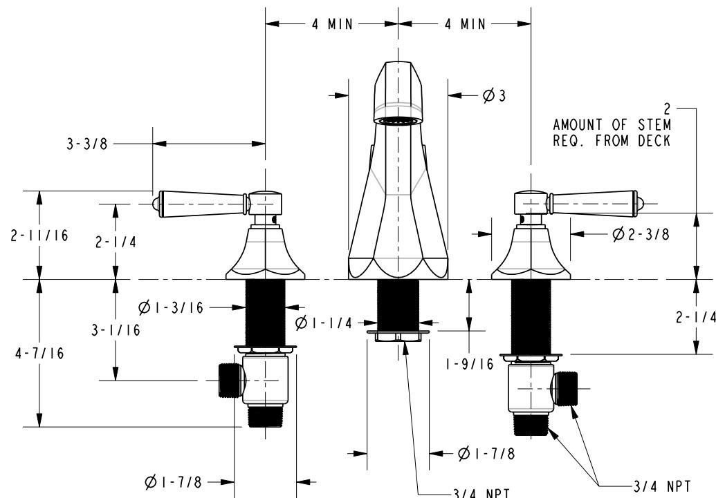
DIMENSIONS ARE IN INCHES AND AN APPROXIMATION OF A TYPICAL INSTALLATION
