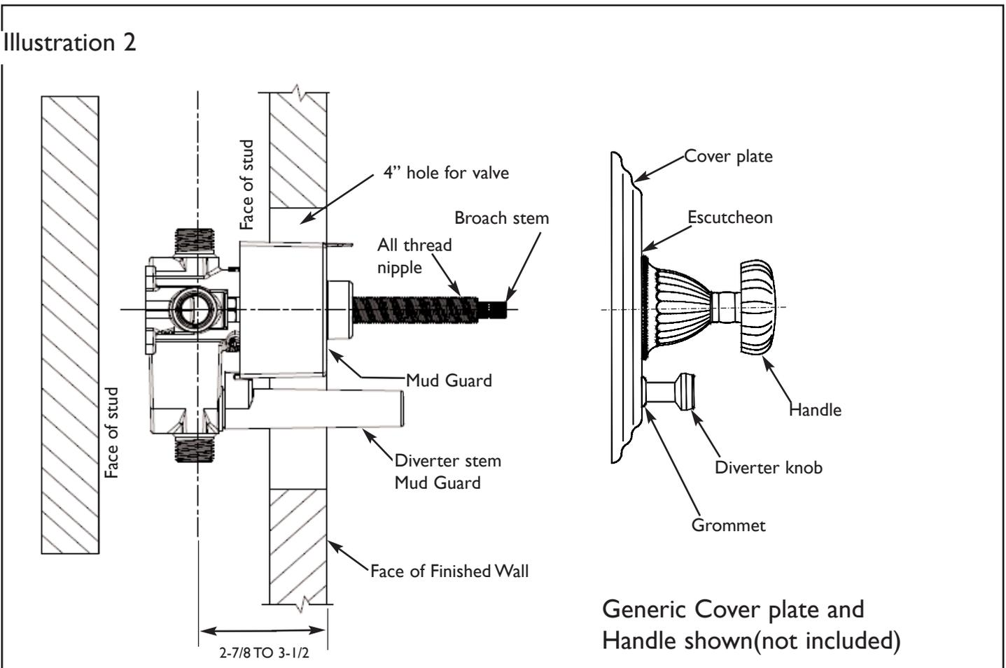
NOTE: Dimensions shown are from the inlet ports to the finished wall.
