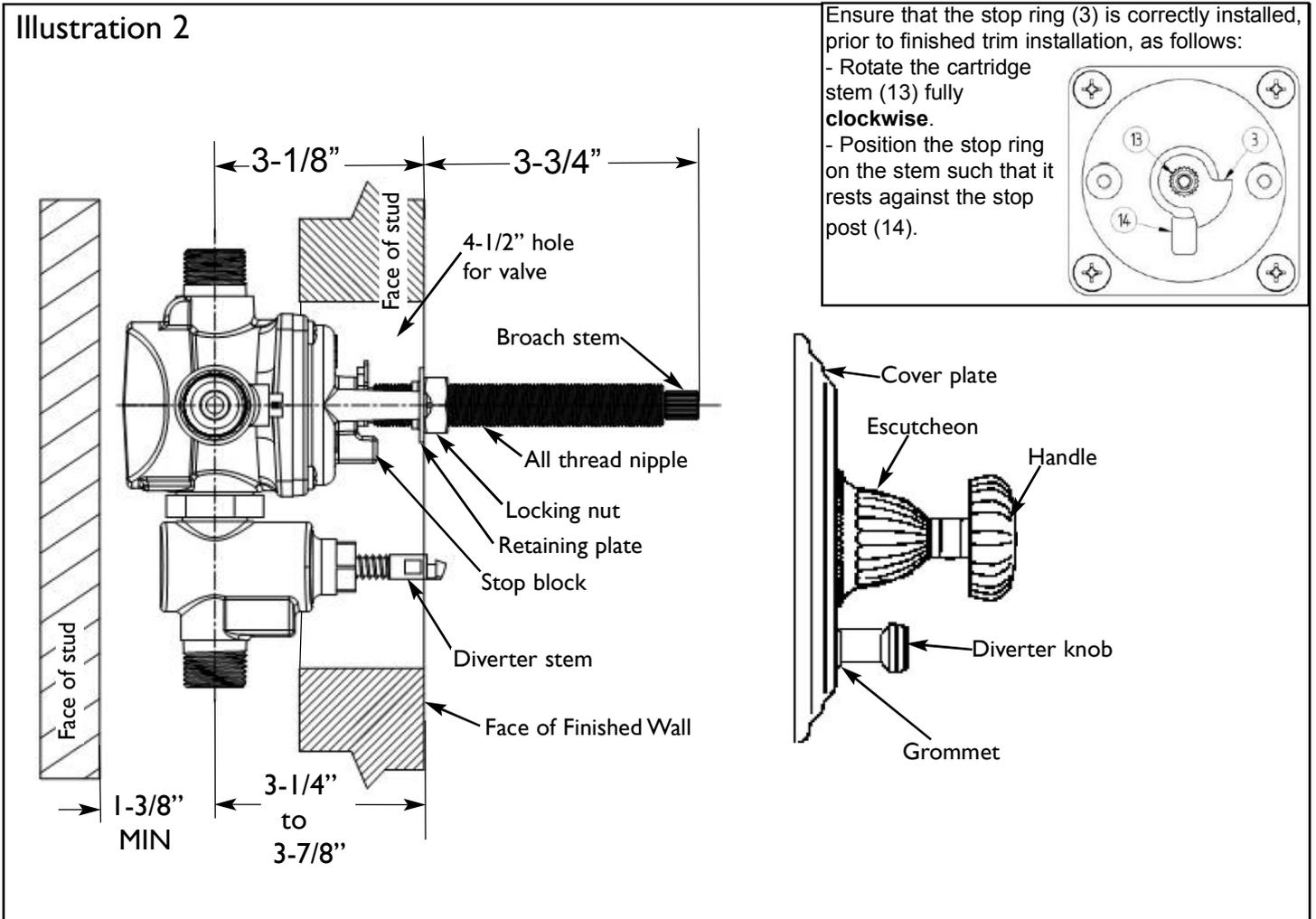
NOTE: Dimensions shown are from the inlet ports to the finished wall.
