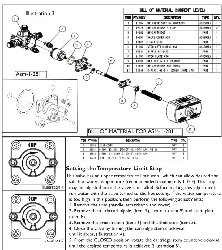
6. Place the limit stop (item 5) on the cartridge stem against the stop block (Illustration 6). Rotate several times to make sure the stop is at the desired temperature setting.
