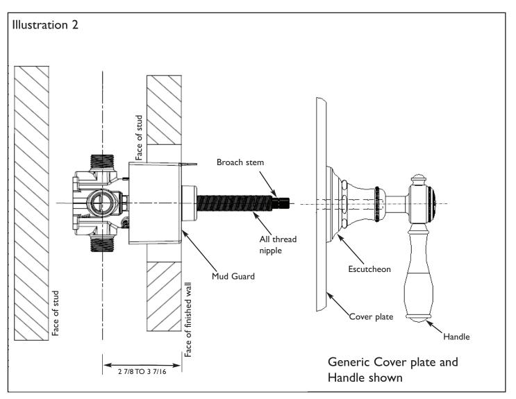
NOTE: Dimensions shown are from the inlet ports to the finished wall.
