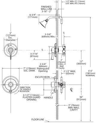
NOTE: This valve is not intended to be used as a shut-off valve. To prevent the potential of cross flow, check valves must be integral to the supply valve or installed in both hot and cold water supply lines.
