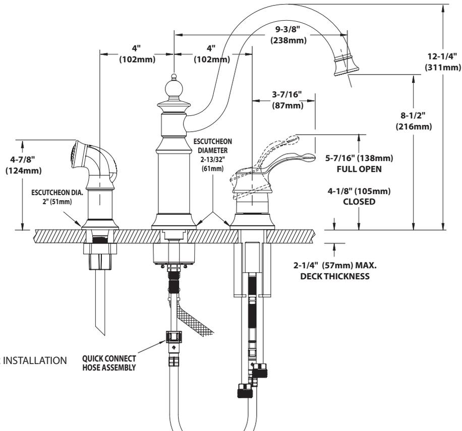
**NOTE:** MINIMUM DIA. HOLES FOR INSTALLATION
