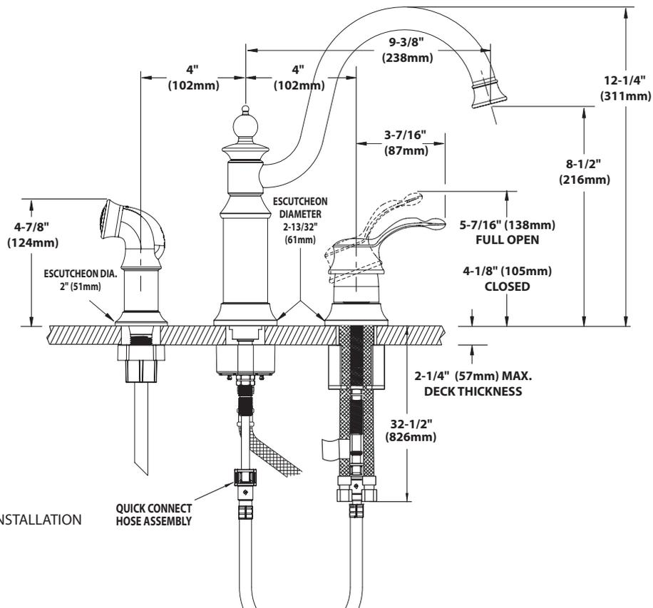
**NOTE:** MINIMUM DIA. HOLES FOR INSTALLATION
