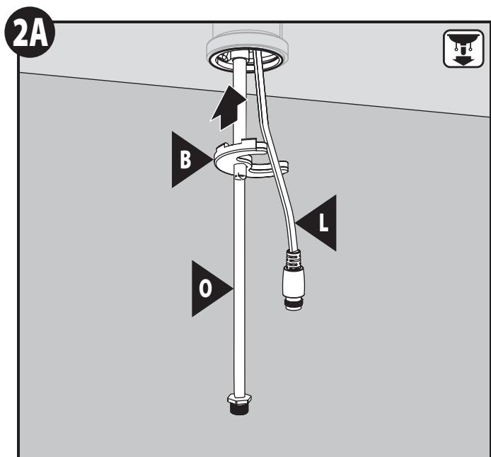
Install Mounting Plate (B) onto mounting shank. Ensure not to pinch Spout Connection (L) with bracket.
