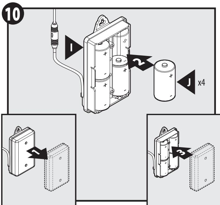
Insert 4 D size Batteries (J) into Battery Box (I). Re-install cover.
