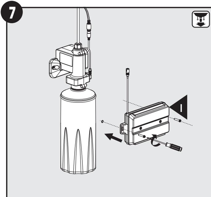
Mount Battery Box (I) to wall and secure with screws until flush with wall.
