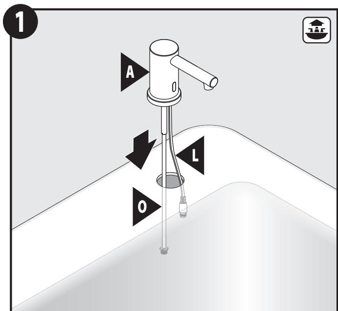
Install Spout (A), Spout Connection (L), and Soap Line Connection (O) into sink opening.
