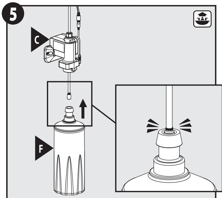
Take Bottle (F) and attach it to connection from Control Box (C). Bottle should click/snap onto connection. Gently tug bottle to test engagement.
