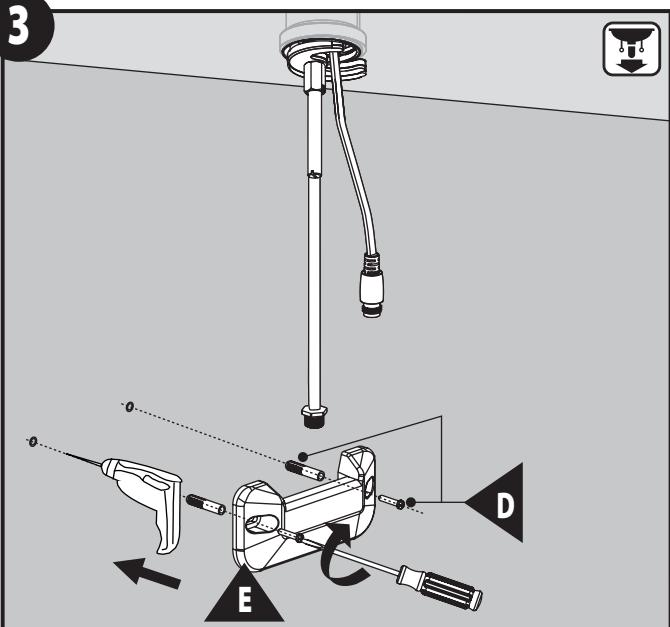
Measure the distance of mounting holes from Mounting Bracket (E). Use that measurement for pre-drilling holes into wall. Mark locations on wall and drill. Using a hammer, tap Wall Anchors (D) from kit. Install Mounting Bracket (E) and secure with Mounting Screws (D) from same kit.
