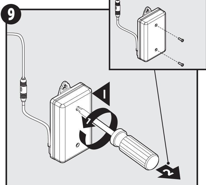
Use a screwdriver to loosen and remove cover of Battery Box (I). Set aside for re-installing.
