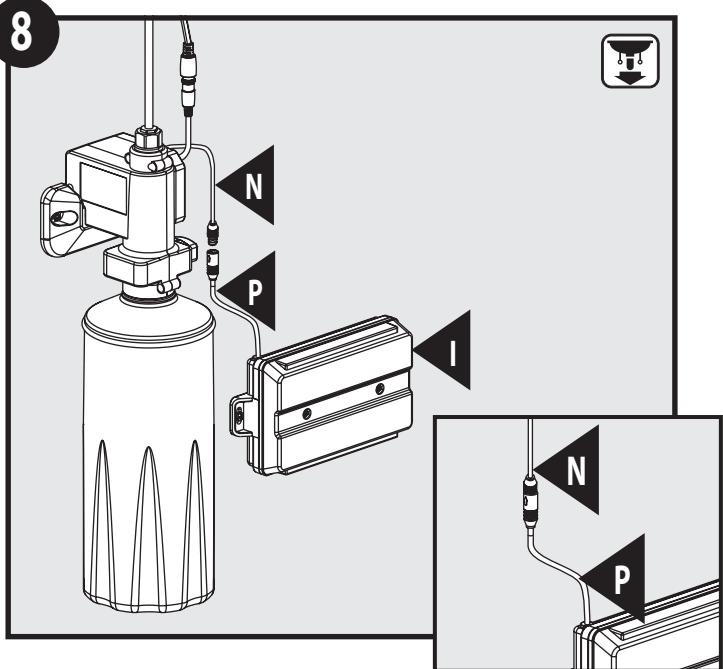
From Battery Box (I), pair the Battery Box Connection (P) to Power Connection (N). Ensure both are fully connected to each other.
