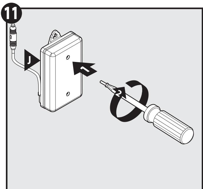
Secure cover to Battery Box (I) with screws.
