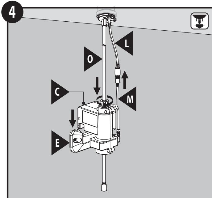
Install Control Box (C) onto ledge opening of Mounting Bracket (E) until it fully rests. Attach Soap Line Connection (O) to Control Box (C) and tighten. Pair the Spout Connection (L) to Control Box Connection (M). Ensure both are fully connected to each other.
