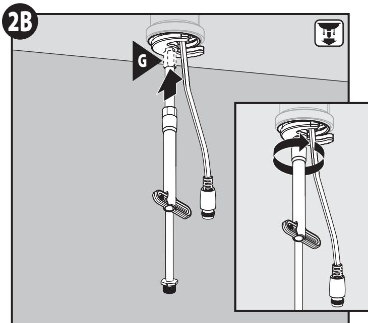
Secure bracket with Mounting Nut (G). Hand tighten, then using supplied Mounting Tool (H), make the final tightening.
