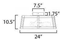
ITEM# LAMPING DIMENSIONS 61022 120V, (4) x 7.25W, 29W Total, LED 3000K D24" X 10.5"H 3,400 2,2
