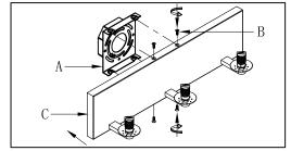
Step.3: Place the fixture body(B) against mounting bracket, Align the two holes of the mounting bracket and fixture body, then tighten the screws(C).
