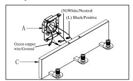
Step.2: Wire fixture to wires in outlet box. Green copper wire is for ground. And carefully position all wires inside the outlet box.
