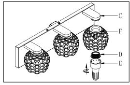
Step.4: Position Glass(F) onto the socket of fixture body(C), then secure with socket ring(D) with Glass (F) onto Fixture body(C) by using spanner(E).
