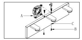
Step.3: Place the fixture body(C) against mounting bracket, Align the two holes of the mounting bracket and fixture body, then tighten the screws(B).
