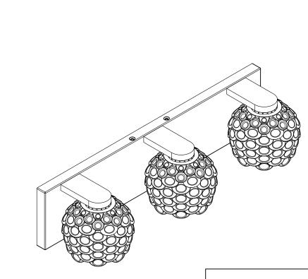
This fixture is designed to dim with an Electronic Low Voltage dimmer. Dimming levels will vary by dimmer.
