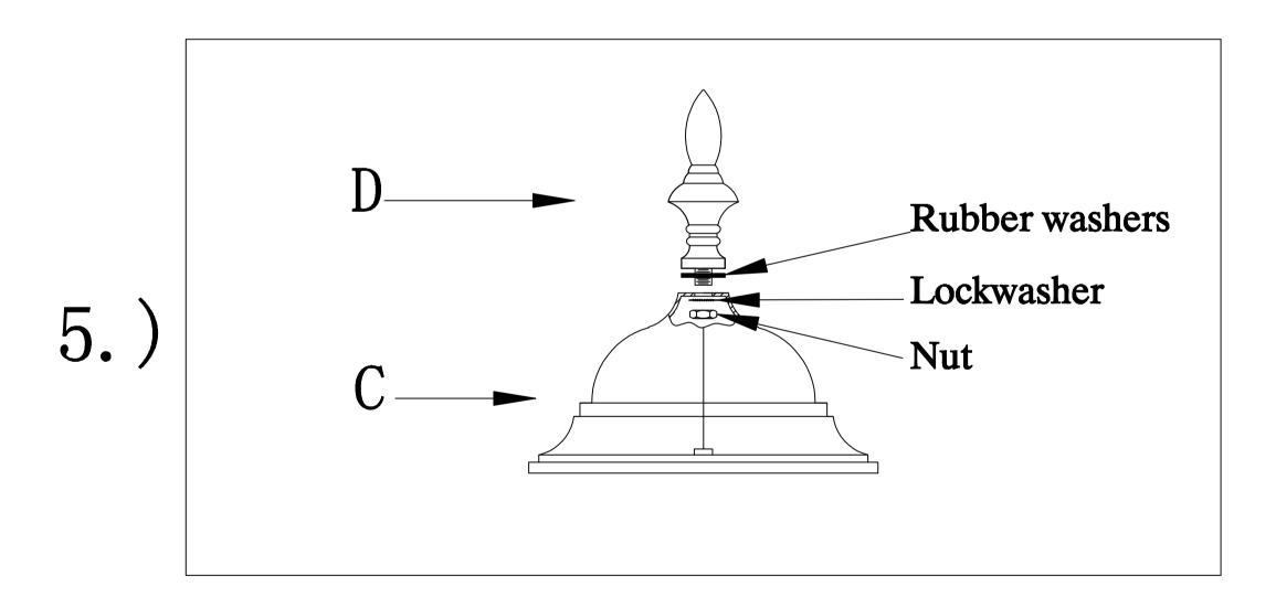
Step.5: Install the finial(D) into the cover(C), using the nuts
