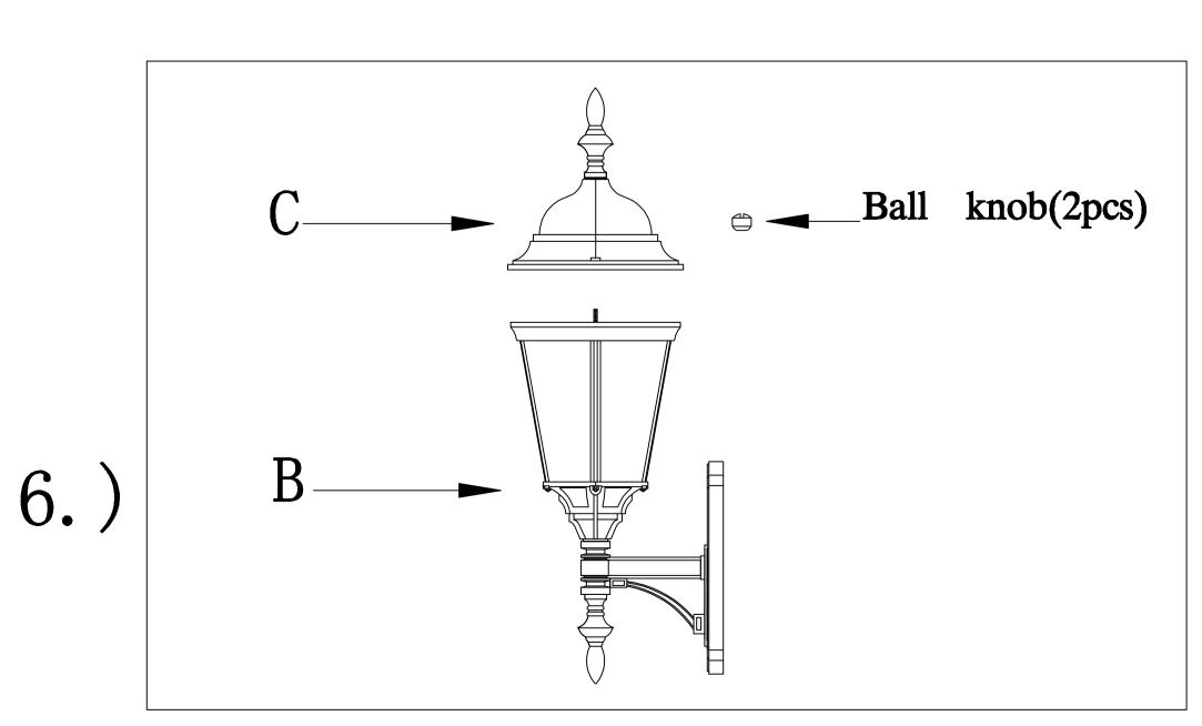
Step.6: Install cover(C) to fixture, using ball knobs.
