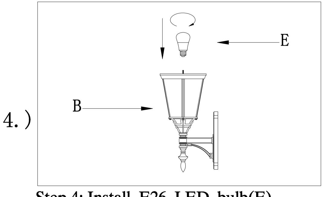
Step.4: Install E26 LED bulb(E)
