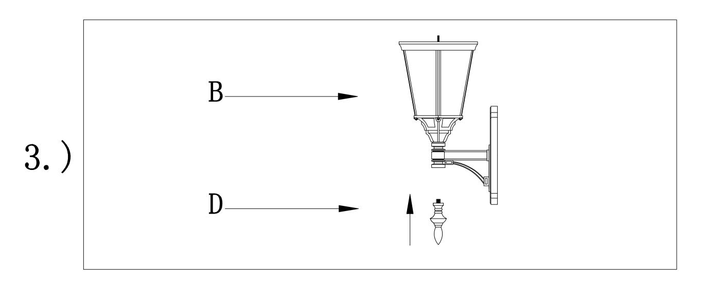
Step.3: Install the finial(D) into the fixture(B)
