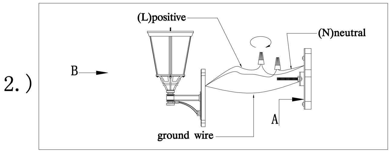
Step.2: Attach back plate to mounting bracket and tighten ball nuts so fixture meets wall. Caulk fixture where back plate meets the wall with silicone sealant.
