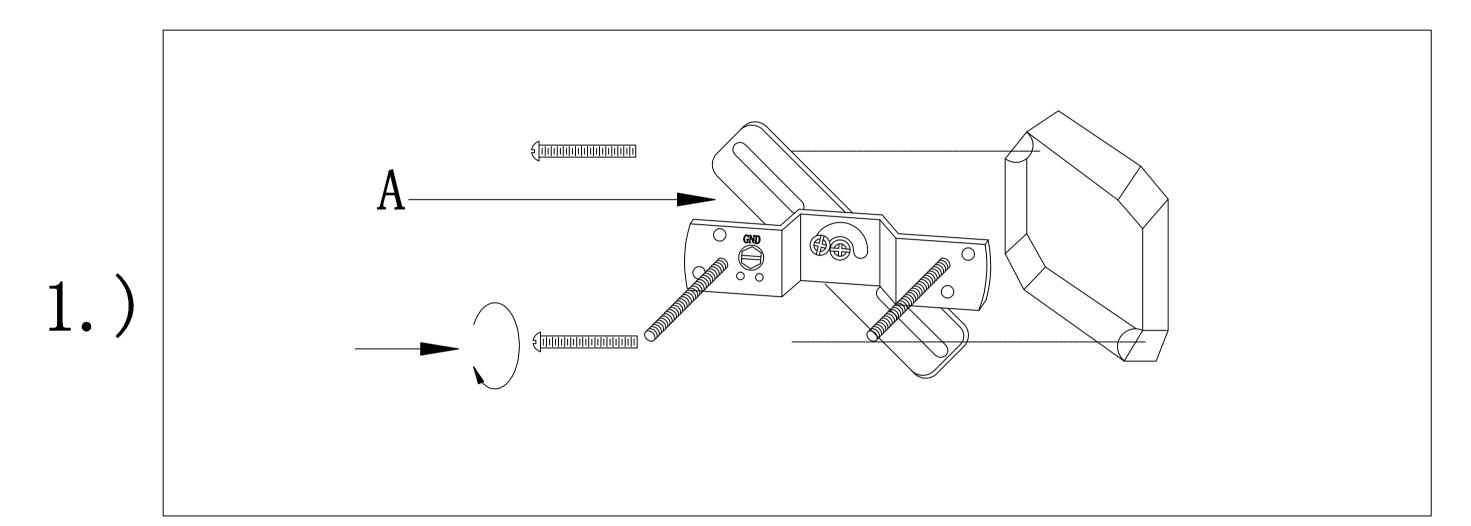
Step.1: Remove mounting bracket from fixture(B) and install to electrical box. then wire fixture to wires in outlet box. Copper wire is for Ground.
