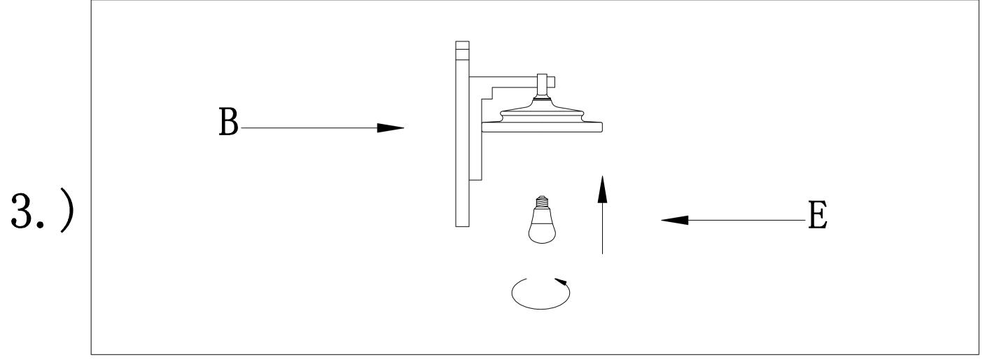
Step.3: Install E26 LED bulb(E)
