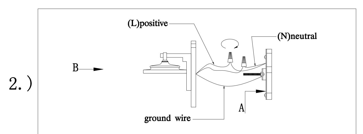
Step.2: Attach back plate to mounting bracket and tighten ball nuts so fixture meets wall. Caulk fixture where back plate meets the wall with silicone sealant.
