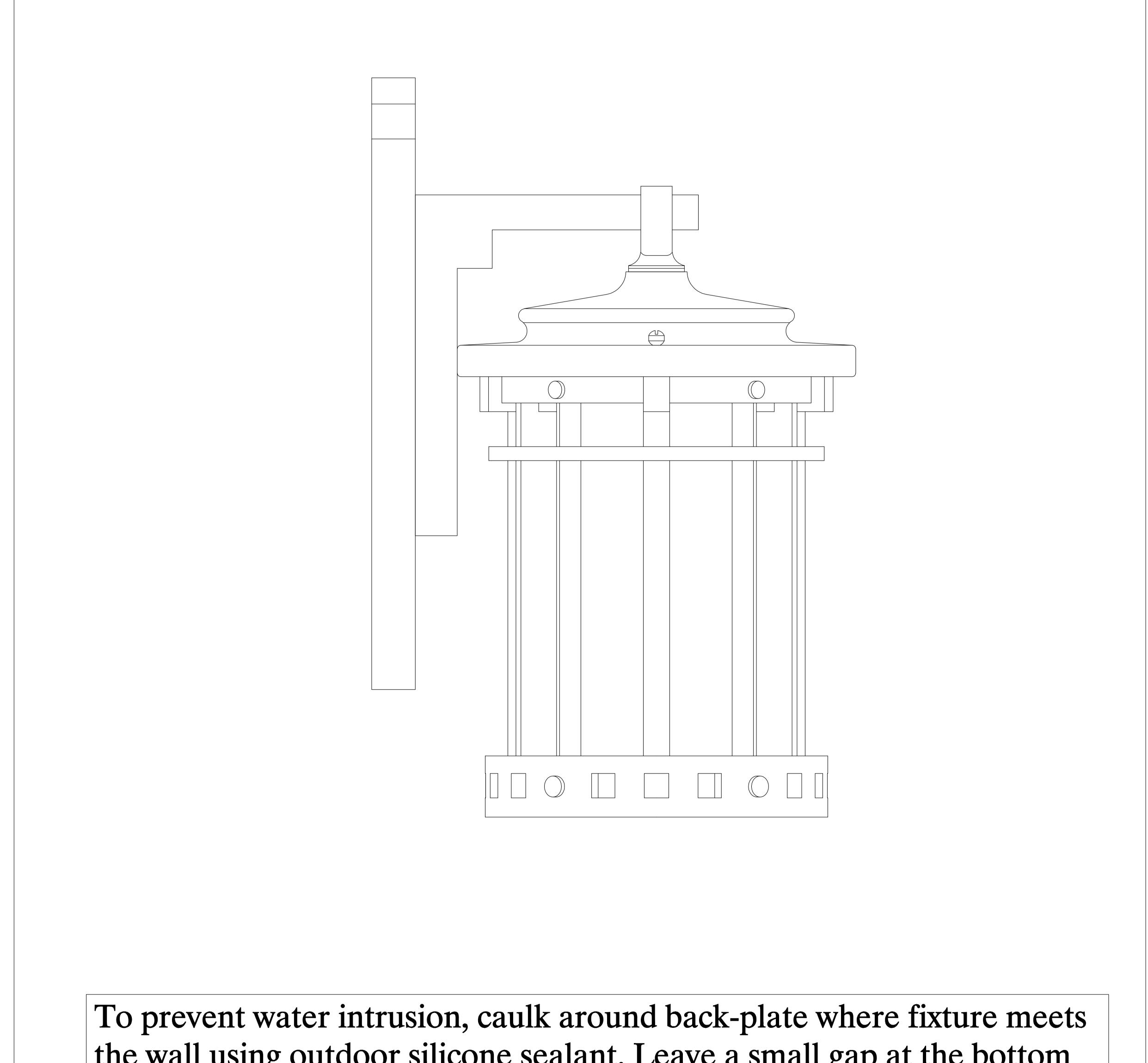
the wall using outdoor silicone sealant. Leave a small gap at the bottom to allow moisture to exit.
