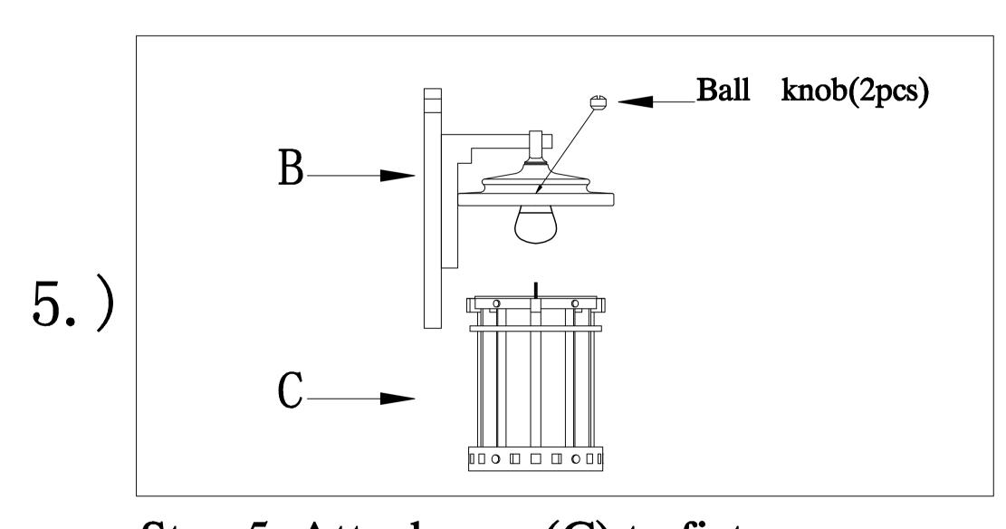
Step.5: Attach cage(C) to fixture, using ball knobs.
