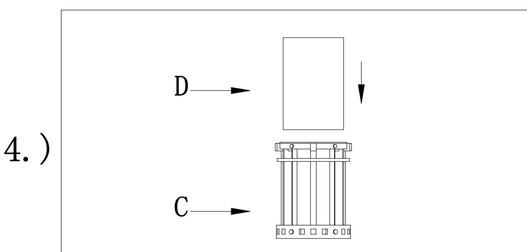
Step.4:Install the glass shade(D) into the cage(C)
