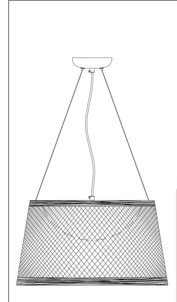
The fixture is designed to dim with a standard Triac forward phase dimmer. Dimming levels will vary by dimmer.
