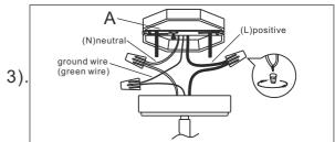
Step.3: Wire fixture to wires in junction box. Copper wire is for Ground.
