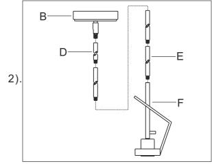
Step.2: Slip first stem section (E) along wire and thread into top of main fixture body (F). Repeat for assembly stem (D) and canopy (B).
