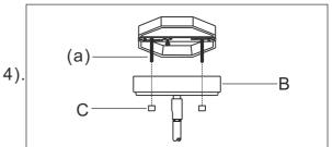
Step.4: Raise canopy (B) over screws (a) and secure with finials (C). Install light bulb. Place glass (H) over the socket, and then secure glass with screw (G).
