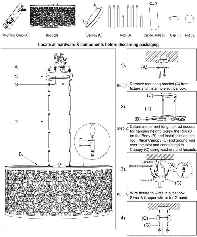
Step.4: Install body (B) to bracket (A) and tighten nut (G) on the canopy (C) to secure. Place the Candle Tube (E) and Cap (F) onto the socket, Install light bulb.
