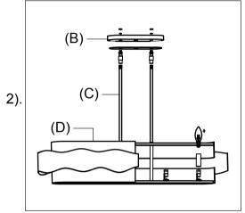
Step.2: Determine correct length of rod needed for hanging height. Screw the Rod (C) on the Body (D) and Canopy (B).
