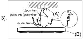
Step.3: Wire fixture to wires in outlet box. Green wire is for Ground.
