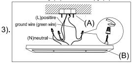
Step.3: Wire fixtures to wires in outlet box. Silver wire is for ground.
