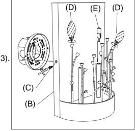
Step.3: Install body (B) to the outlet box and secure with screw(C). Install crystal (D) on the arm. Insert bulb (E) in the socket.
