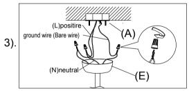
Step.3: Connect the white and black driver wires to the fixture wires with terminal block, connect the white driver wire to the neutral power line wire and the black driver wire to the hot power line wire with wire nuts (see wiring diagram for details). Note: The positive fixture wire is marked by white tracer.
