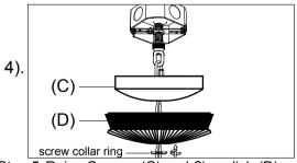
Step.5: Raise Canopy (C) and Glass dish (D) to ceiling and secure with screw collar ring. Place the Cap and Glass dics onto the nipple and secure with the glass finial (F), install Glass (G) as shown on the drawing. Place the Socket cover (H) and Glass Bobeche (I) over the socket and Install light bulb.
