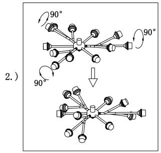
Step. 2: The fixture is packaged flat, Turn the arm 90 degrees clockwise for correct configuration.
