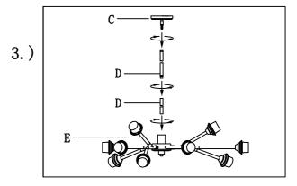
Step. 3: Run wire through stems (D) and combine stem lengths to meet desired mounting height.
