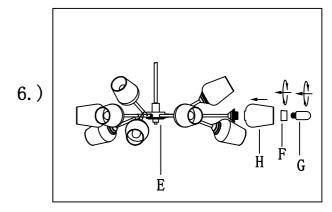
Step. 6: Use socket ring (F) to secure the glass(H), then install the bulb(G).
