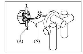
Step 2: Then wire fixture to wires in outlet box. Copper wire is for Ground. Install lamp body to mounting bracket using two screws on side.
