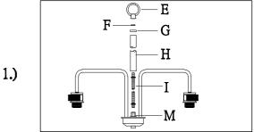
Step. 1: Attach the tube(H), metal cap(G) and finger ring(F) to the nipple(I), then secured by loop(E) till tighten
