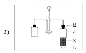
Step .3: Attached the glass(J) and metal shade(K) to the socket(M), then secured by socket ring(L)
