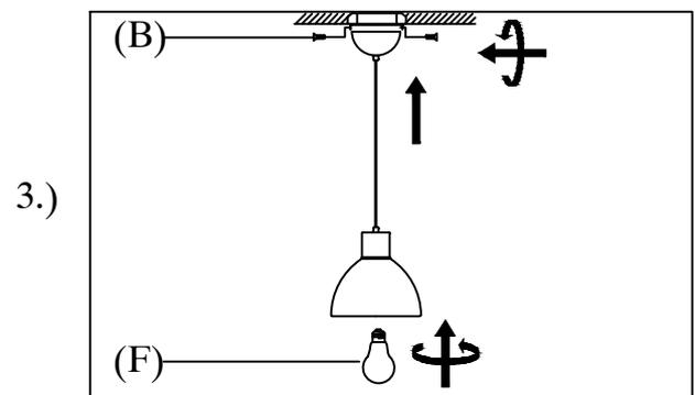
Step3 :Install fixture to bracket and tighten screws at the ends of the canopy to secure. Install bulb into socket.
