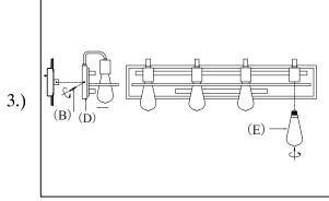
Step3: Install lamp body to back plate using two screws on side. Install bulb into socket.
