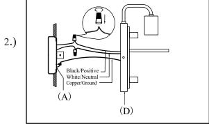
Step2: Wire fixture to wires in outlet box. Copper wire is for Ground.
