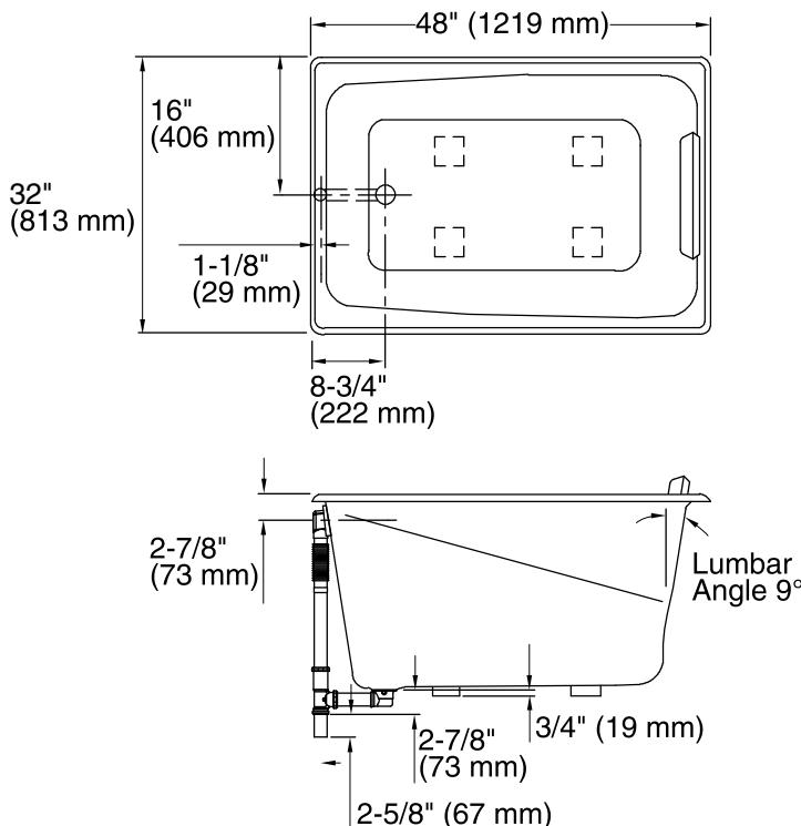
No change in measurement if connected with drain illustrated. (K-7256)
