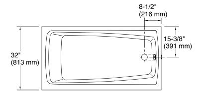
No change in measurements if connected with drain illustrated. (K-7213)
