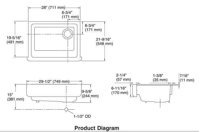
WHITEHAVEN<sub>®</sub> UNDER-MOUNT SELF-TRIMMING<sub>®</sub> APRON FRONT KITCHEN SINK Page 2 of 2 1176676-4-**B**
