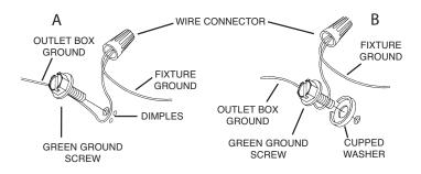
5) Make wire connections. Reference chart below for correct connections and wire accordingly.
