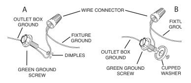
3) Make wire connections. Reference chart below for correct connections and wire accordingly.
