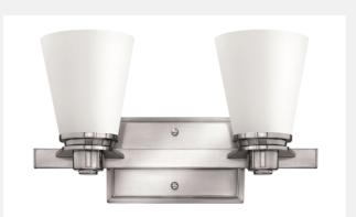
AVON 5552BN-LED BRUSHED NICKEL WIDTH: 14.5" HEIGHT: 8.0" WEIGHT: 4.0 LBS METAL MATERIAL: GLASS: ETCHED OPAL BACKPLATE WIDTH: 7.3" BACKPLATE HEIGHT: 4.5" SOCKET: 2-15W LESM-100 \*INCLUDED LED INFO: LUMENS: 1100 COLOR TEMP: 2700k CRI: 90 LED WATTAGE: 15w INCANDESCENT 100w EQUIVALENCY: DIMMABLE: YES EXTENSION: 6.3" TTO: 5.8" **CERTIFICATION:** C-US DAMP RATED VOLTAGE: 120V UPC: 640665555479 INSTALL OPTIONS: UP AND DOWN
