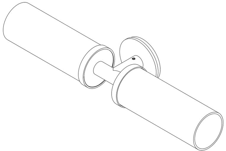
\* *Installation Note (Electrician/Wall-finisher): This light uses a non-standard size backplate. This light is designed to be installed onto a raised cover plate (also known as a round plaster ring or round raised mud ring) attached to an electrical box installed pre-drywall stage. Use two no. 8 tapped holes on 2-3/4" centers. Maximum diameter of finished opening is 3-3/8".*
