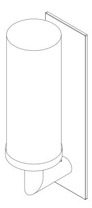
\* Installation Note (Electrician/Wall-finisher): This light uses a non-standard size backplate. This light is designed to be installed onto a standard vertically installed switch box. Maximum width of finished opening is 2-1/2".
