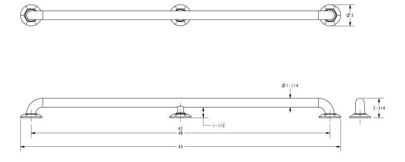
$\overset{\bullet}{\underset{}_{\overset{\bullet}{\overset{}}}}$  meets or exceeds astm F446 standards and conforms to ADA guidelines.
