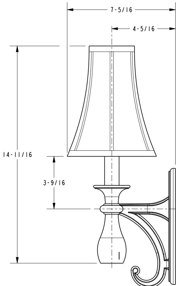
DIMENSIONS ARE IN INCHES AND AN APPROXIMATION OF A TYPICAL INSTALLATION
