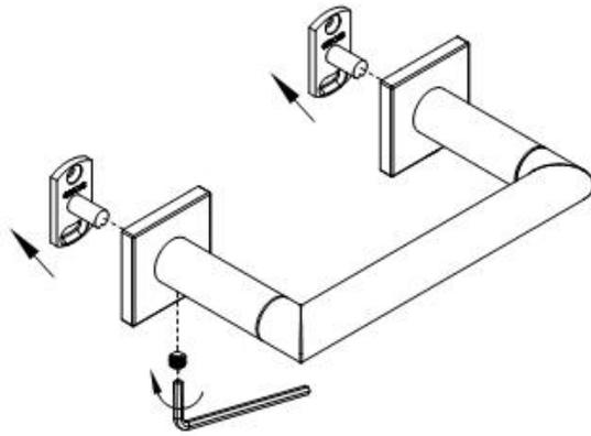
② ALIGN MOUNTING BRACKETS AND MARK LOCATION
